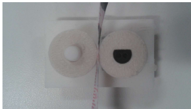
Two roller wheels with tape positioned between.
