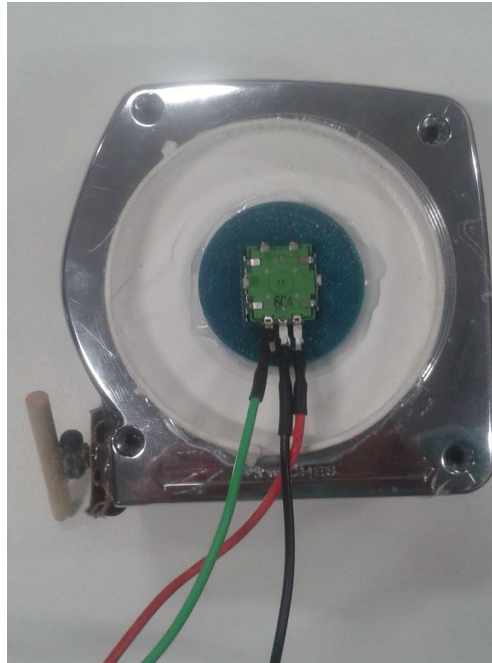
Outside casing of the hub-mount encoder model. The encoder is centered on the spool.
