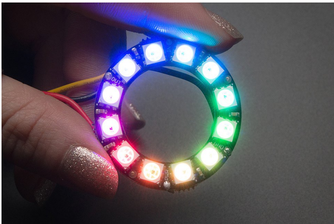
Figure 7: The LED ring that we selected from Adafruit
